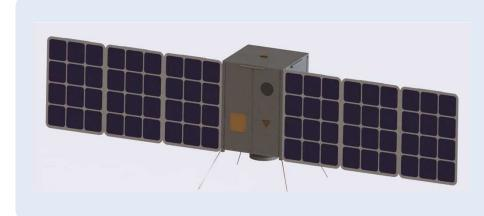
12U Cube Satellite Design with deployable solar panels
